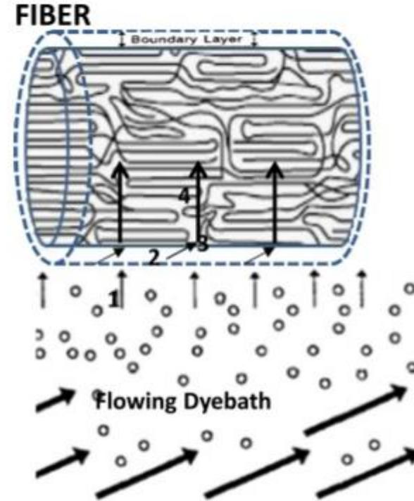
Dyeing and more particularly dye transport through PET fibres is function of both diffusivity and solubility of the dye in the PET fibre[Slark, 1999 ].
