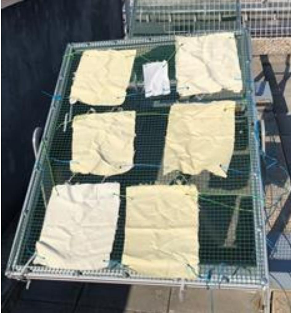
*Samples washed during 3 hours at room temperature (to simulate effect of intense raining)*
